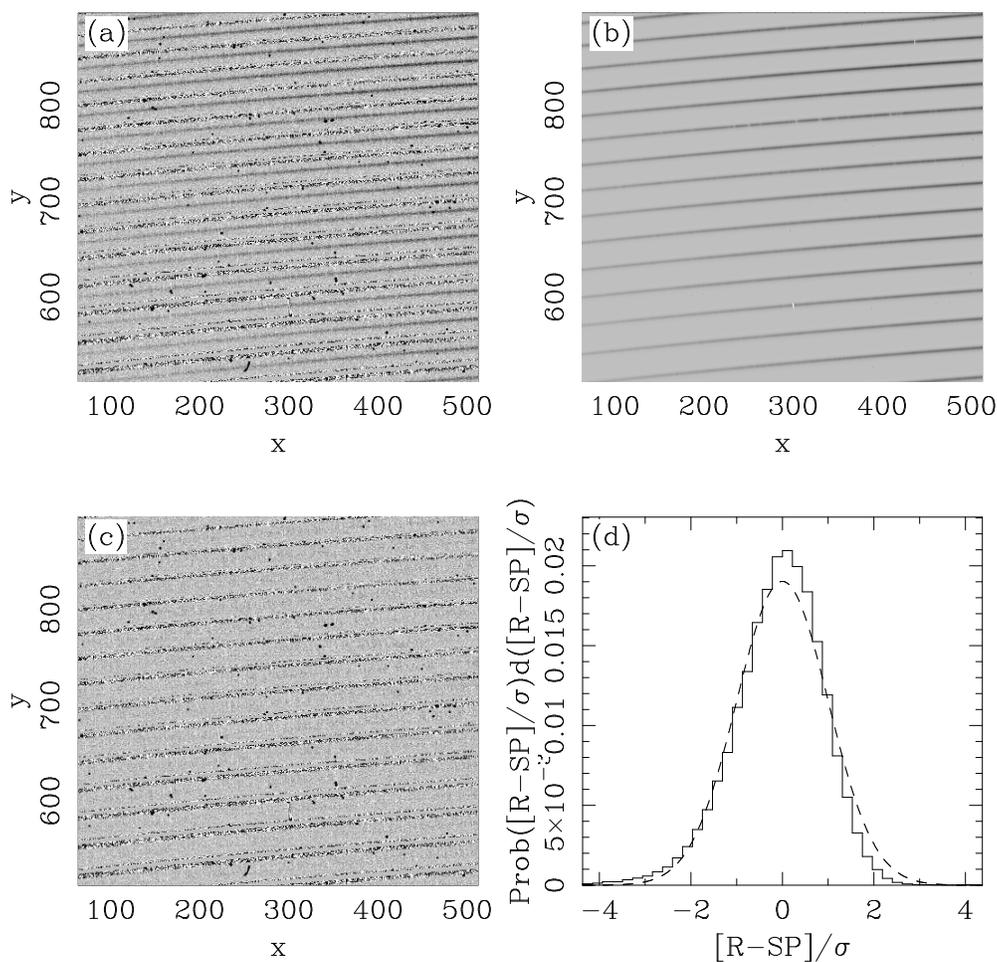
Fig. 5.— Same as in Figure 3 but for a subsection of data on a faint source. For these data the fitting for  $S$  was performed using six exposures. The distribution of residuals is skewed slightly and the small non-Gaussiannity results from noise being dominated by the read noise. The bi-weight estimators for location and scale indicate a 4% deviation from the expected values for the first and second moments of the distribution.
